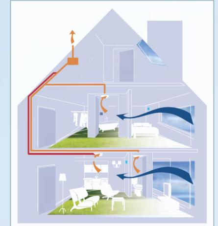
The diagram illustrates a typical "System 3" central extract duct layout, focusing on the 'Best Practice' that the toilet extract is separate to, or positioned in line between the kitchen extract and the extract unit.
